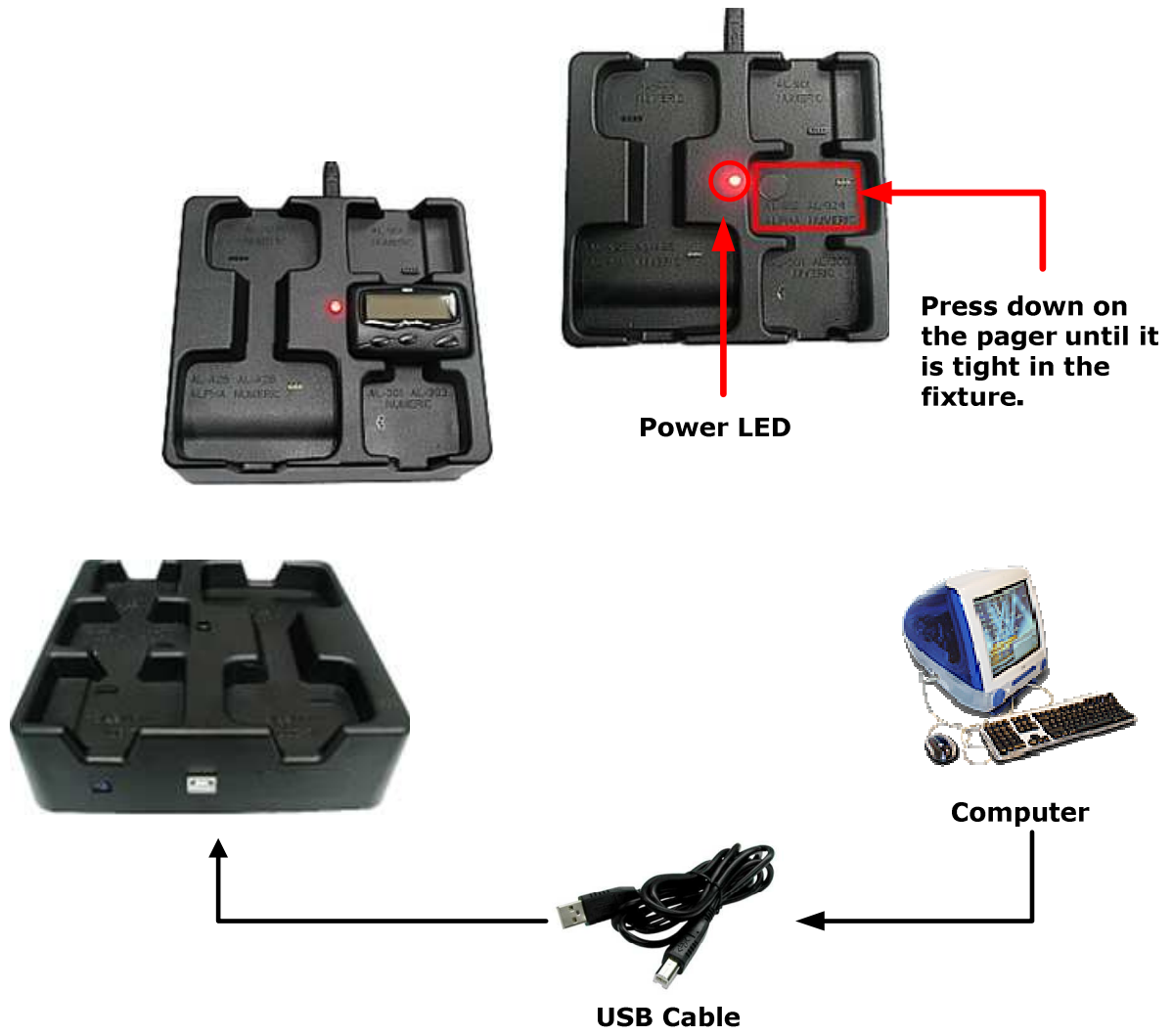
Figure 1 Programmer Hardware Connections
